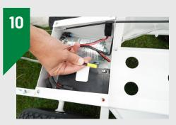
Attach the yellow plug to the battery. Replace the lid and secure using supplied bolts and allen key.
