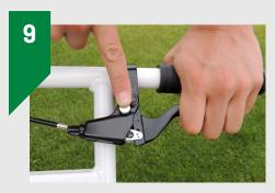
To keep the discs off the ground permanently press the button on the handle while squeezing it.
