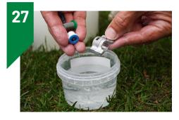
Clean the nozzle and filter and place all items in a small container filled with water or add our Selectline Cleaner.
