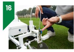
Turn the ball valve to vertical position.
