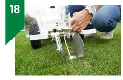
As soon as paint comes out, return the ball valve to horizontal postition.
