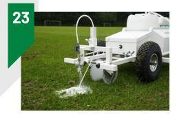
Turn the ball valve to vertical position and rinse the tubes by pressing the switch.
