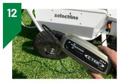
Connect the charging plug to the machine and the charger to a 220V socket. An indicator light tells you the charge level. The battery is fully charged when the '5' lights up green.
