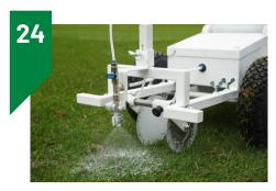
Return ball valve to horizontal position to rinse spray head and nozzle.
