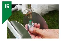
Put the nozzle in the nozzle holder, place the flat seal firmly on top of it and finally the filter. Then screw the nozzle holder onto the spray head.
